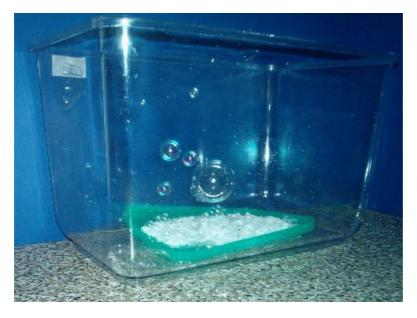
Carbon dioxide is more dense than, and descends in normal air. Because the air filled bubbles are less dense, they float on the invisible layer of carbon dioxide in the aquarium. Helium filled balloons float in air for exactly the same reason, except that helium is less dense than air. Any substance (or object) will float when immersed in a fluid (ie gas or liquid) if the substance (or object) is less dense than the fluid.
